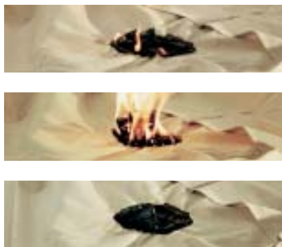
With Trevira CS safety fabrics the effect is that a fire - perhaps from a burning newspaper - self-extinguishes.
